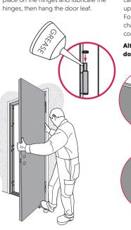
frame is vertical. For double doors, the hinge side of the active door must be vertical.
